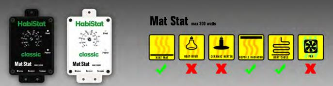
The **Mat Stat** is an on / off switching thermostat, that can be used for controlling the temperature of heat mats and other low powered heaters up to a maximum load of 300 Watts. Put simply, the thermostat switches a heater on full power until the set temperature is achieved and then it switches the heater off completely until the temperature drops below the set value, when the cycle starts over again.
