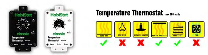
The **Temperature Thermostat** is an on / off switching thermostat, that is ideal for controlling heat mats, and other low powered heaters up a maximum load of 600 watts. Put simply, the thermostat switches a heater on full power until the set temperature is achieved and then it switches the heater off completely until the temperature drops below the set value, when the cycle starts over again.
